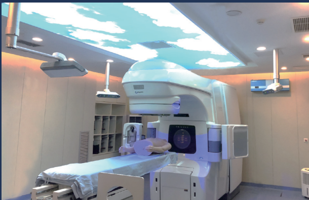
Klarity SGRT System with three cameras solution for Varian Trilogy
