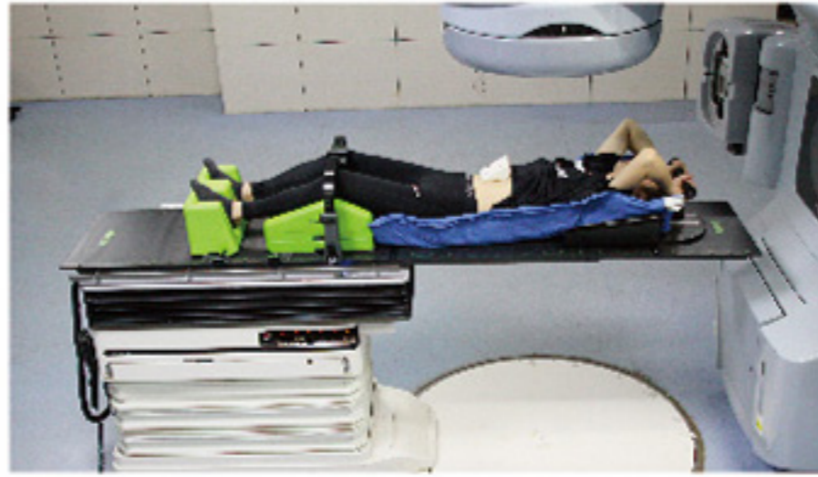
System B: TRiNiTi® 6 DoF Robotic Couch for high precision patient position corrections in 6 degrees of freedom
